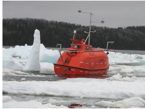
Testing a lifeboat in pack ice off Newfoundland TK at the helm – headway was possible in 7/10s or less but needed a lot of work. Boat rigged for video and other monitoring
