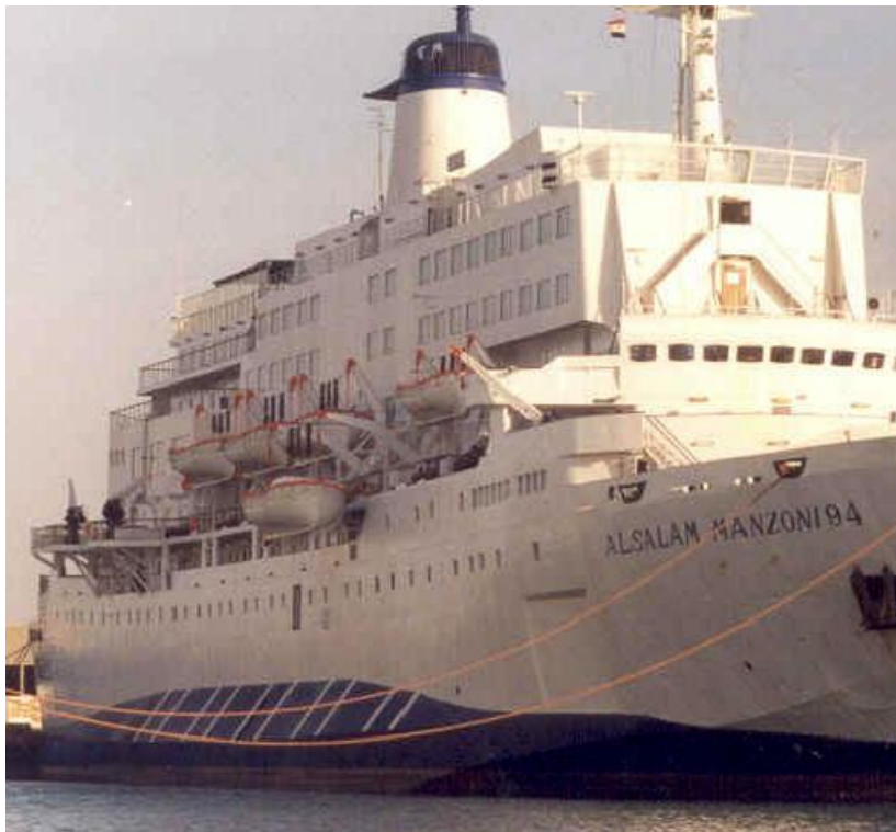
The blisters on the side of the AL SALAM MANZONI 94 , similar to those on the BOCCACCIO
