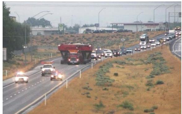
At Pasco the turbine was lifted on to a long-haul transport trailer for carriage to Coulee City, upstream of the Grand Coulee Dam, a distance of about 235 kms along Washington State highways.
