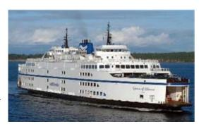
The *Queen of Alberni* was originally built to handle overheight vehicles. In 1984, the ship was stretched and lifted, gaining an upper car deck for non-overheight vehicles, leading to a new vehicle capacity of 292. In 1999, the ship underwent another refit in Victoria. This recent extensive upgrade involved significant mechanical and safety improvements as well as new and improved passenger amenities. The upgrade, preparing the vessel for another 20 years of service, includes:-
