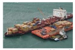
About 4,000 tons of bunker oil was safely removed. Then a barge equipped with two cranes lifted off the containers, landing them on shuttle barges. By the beginning of March all 860 containers had been removed from the ship's deck. It then took until mid-May before all containers had been discharged from the ship. The salvage crew involved a team of 40 people. Subsequently equipment was brought in to pump water out of various compartments.
