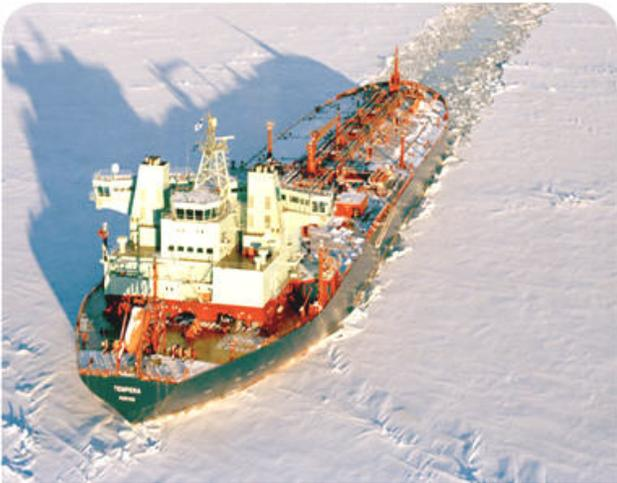
There are tankers and other vessels with the ability to break thick ice when backing into it, as shown here
