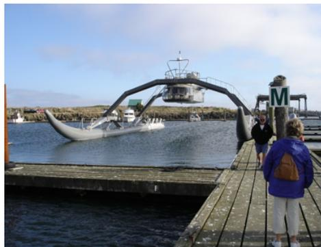
Daddy-longlegs. Rubber pontoons forward with metal tubes aft for the engines and jet drives. What looks like old leaf springs support the legs on which the wheelhouse sits.
