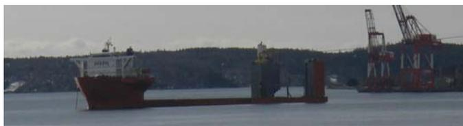
The heavy lift ship *BLUE MARLIN* sits ready to load in Halifax harbour once it sinks its deck under water
