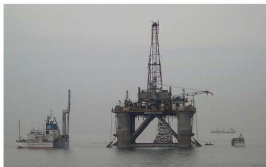
The semi-submersible oil rig *ALEUTIAN KEY* is moved off the deck of the cargo deck of the heavy lift ship *MIGHTY SERVANT II*
