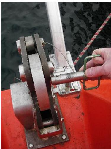
Safety pin being withdrawn from hook and side plates
