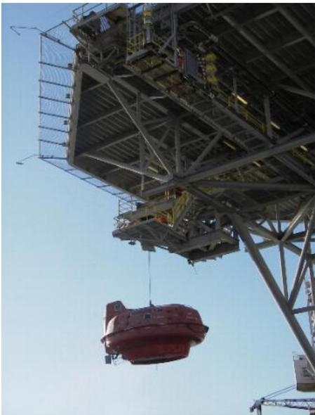
The ability to turn very quickly is an asset as the single fall Whittaker can spin round when being launched
