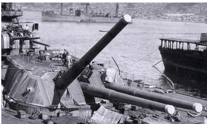
Yamato 18.1" Triple Turret, 2,510 tons Source:
